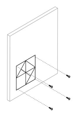
2 Attach one of the bottom quilt panel to the wall using appropriate fasteners for the wall surface material.
