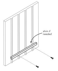
Level and attach a ledger board to your wall using appropriate fasteners for the surface material.
